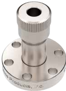
210833 / 1/4 Inch Tube Ultra Torr® Fitting to 1.33 CF Flange
